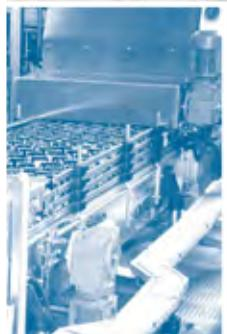
**POSIJET-CANS** SINGULATOR is an air conveyor for empty cans, that singulates them smoothly into a single line at very high filler line speeds.
