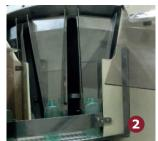
The funnel guides the bottles towards the machine exit, and once there, they are deposited on the exit conveyor. They can exit in two ways: air conveyor belt (3) for flat-base bottles, or in star-wheel with POSIJET air conveyor (4) for bottles with petaloid bases.
