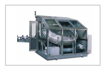
Completely closed cabins made of removable panels and easy-access doors to carry out bottle format changes and for cleaning and inspection work. Available with two types of finish: plastic-coated steel or AISI 304 stainless steel with soundproofing of 80dB(A). Cabins with enhanced soundproofing of up to 75dB(A) are also available.
