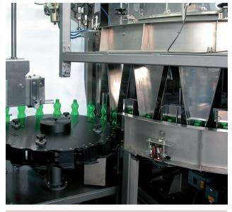
The discharge wheel empties both funnels, the main and the auxiliary one, so that they can be filled again on the next rotation.
