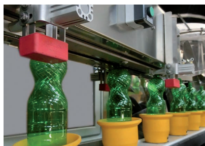
POSITRANS: for bottles with petaloid bottom + POSIJET air conveyor.
