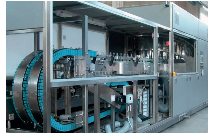
Ionised air Rinser in monobloc with Unscrambler
