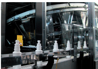
VACUUM CONVEYOR: for bottles with flat bottom.
