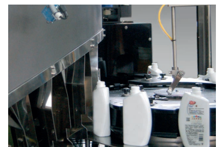
STAR-WHEEL: for special shaped bottles.
