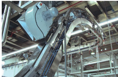
Air Conveyor working vertically
