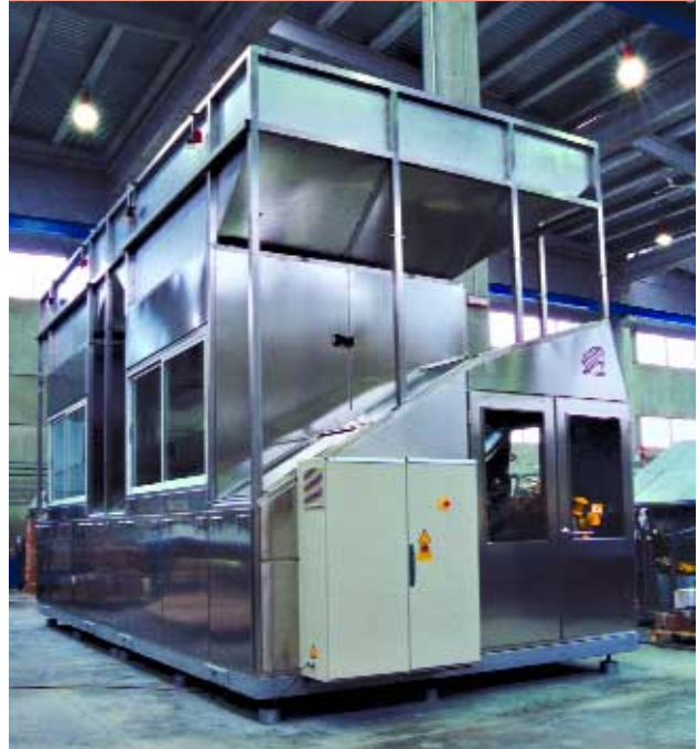
POSISILO Inbuilt onto a POSIMAT unscrambler
